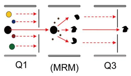
Fig 2: Schematic diagram of multiple reaction monitoring mode by mass spectrometry
